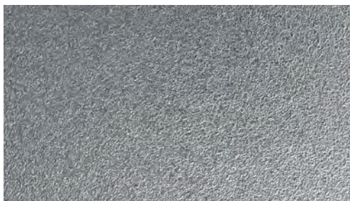
Patterned finishes combine a non-reflective surface effect with good cleanability. Photos: Aperam
